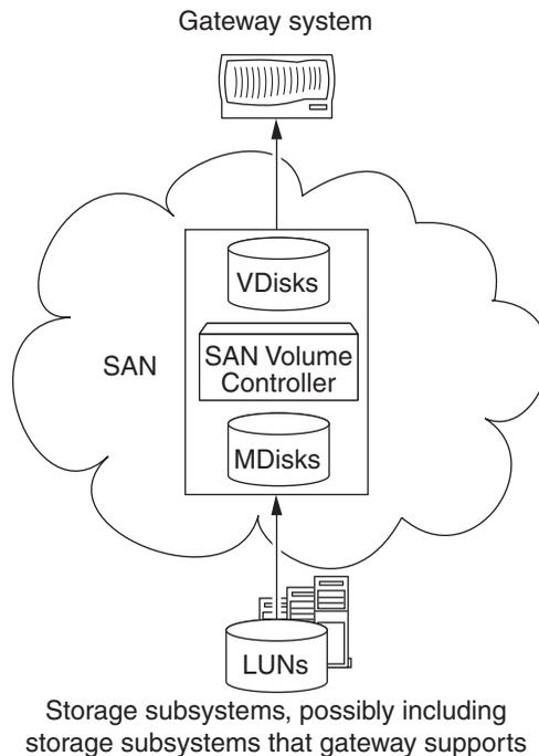
When SAN Volume Controller provides all the storage for the hosts, the storage arrays are all configured to see only SAN Volume Controller as their host. SAN Volume Controller is configured see all the hosts, including the gateway, and presents the storage as VDisks to the hosts.
